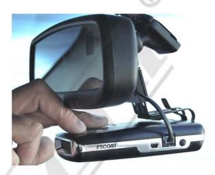
6 - To access the buttons of the RD you will need to gently push downward on the front of the RD with one finger and push the desired button with another finger. Then allow the RD to return to it's original position by gently letting it spring upward. When accessing the buttons, be sure to push the RD downward just enough for your finger to fit between the RD and mirror. Do not push down more than what is needed.
